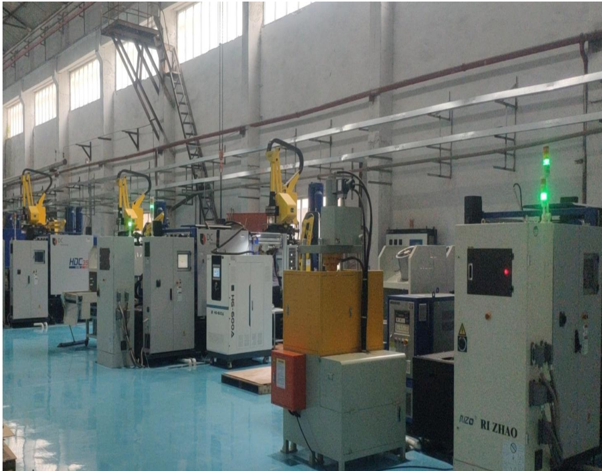
Magnesium, aluminum, and zinc alloy die casting (with vacuum equipment)
